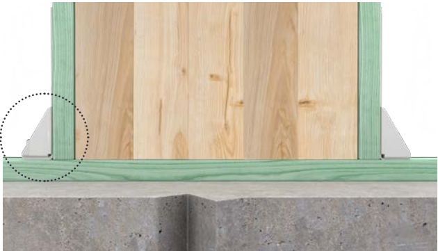
Figure 8. Brackets both outside with single stud wall
